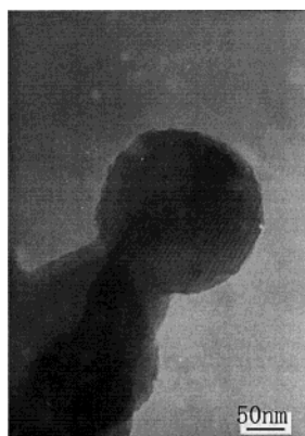
Figure 16. TEM micrograph of the PVAc/silylated MCM-48 nanocomposite prepared by the post-polymerization method.
